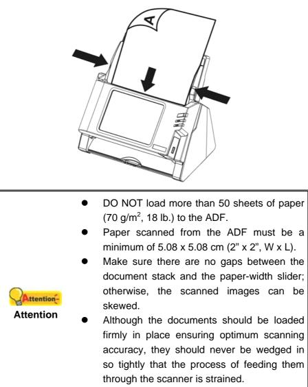
Do not load additional paper into the ADF while the unit is feeding and scanning.
