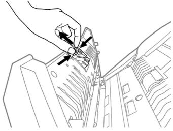
3. Close the panel unit by pushing it back down until it snaps back into place.
