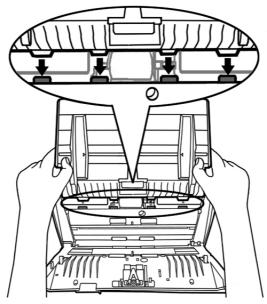
3. Close the panel unit by pushing it back down until it snaps back into place.
