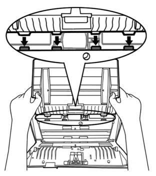
6. Close the panel unit by pushing it back down until it snaps back into place.
