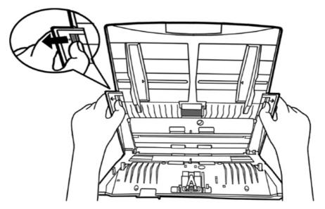
3. Remove the feed roller by pinching both sides of the feed roller and pull it out.
