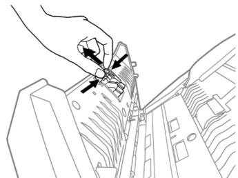
3. Install the new pad module by inserting the tabs on the module onto their slots on the scanner.
