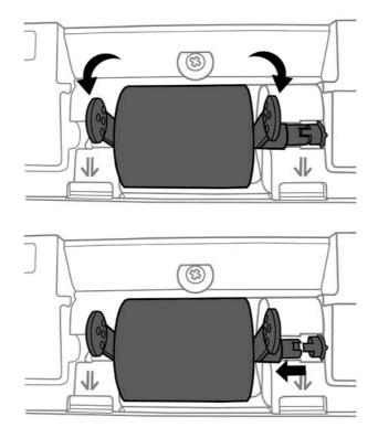
4. Install the new feed roller by aligning and inserting the feed roller onto the roller pitman on the scanner.
