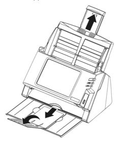
3. Adjust the paper width slider for the paper size you are using. The paper width slider should be gently touching both sides of the documents.
